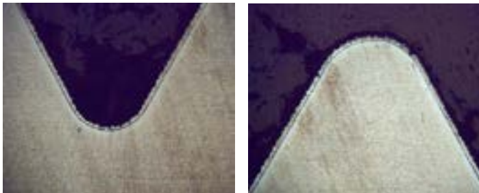
Figure 2. View of TDG coating on the coupling thread when measuring the thickness by the metallographic method: a. socket; b. apex of the tooth
